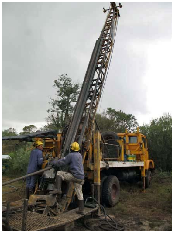
Figure 21: Diamond drill rig at Butiá
