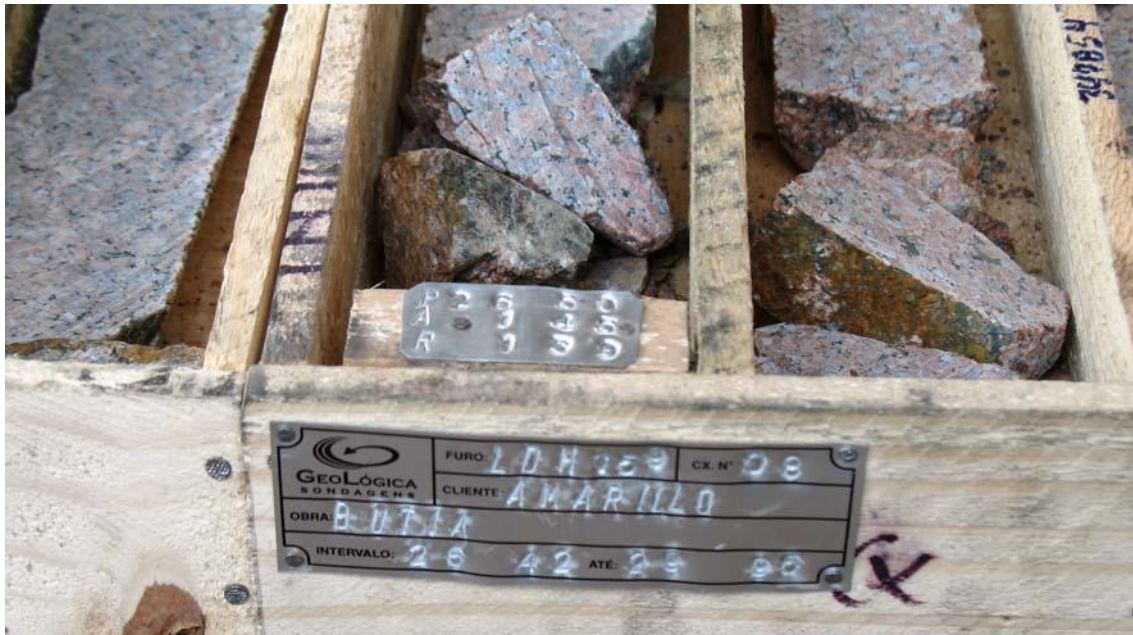
Figure 23: Core boxes clearly marked
