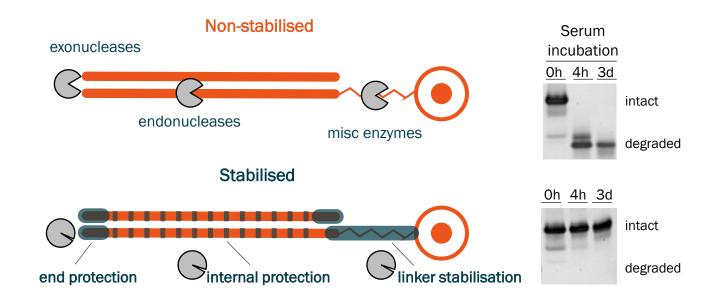
Incorporation of chemically modified nucleotides can protect GalNAc-conjugated siRNA from degradation
