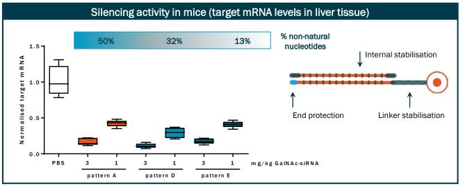
Incorporation of novel chemical modification patterns, end-protecting and linker-stabilising moieties yields robust GalNAc-siRNA silencing in vivo
